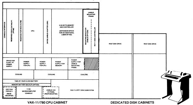
Dual RK07 Disk-Based VAX-11/780 System Configuration
